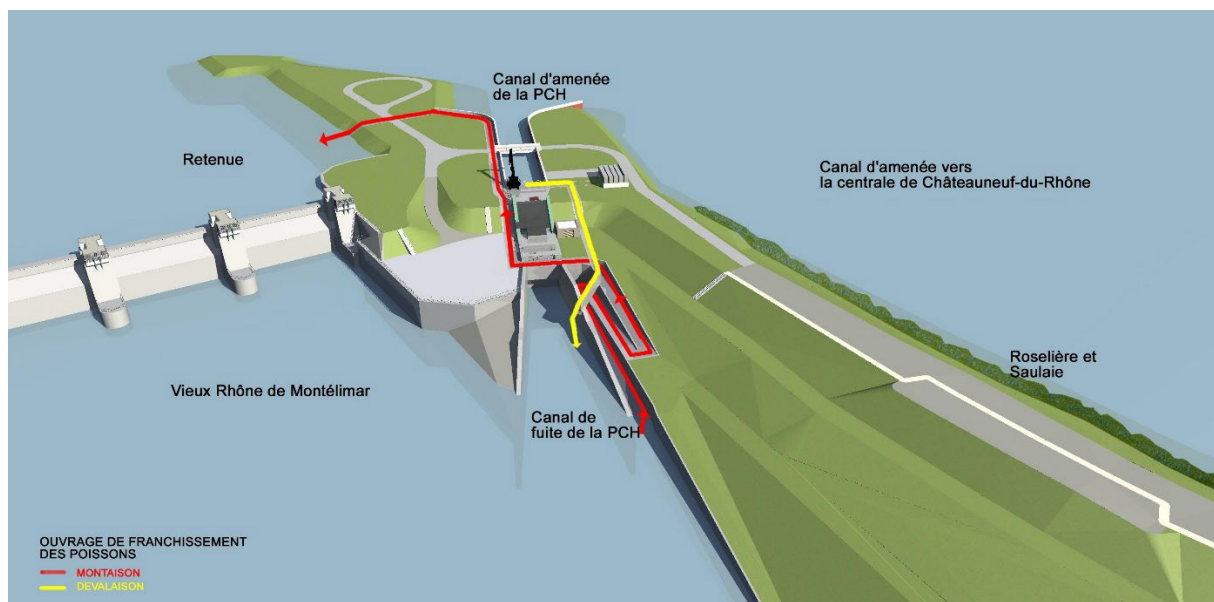
Figure 2. standard installation of CNR on the Rhône River with SHPP and fish ladder – Châteauneuf-du-Rhône dam.
